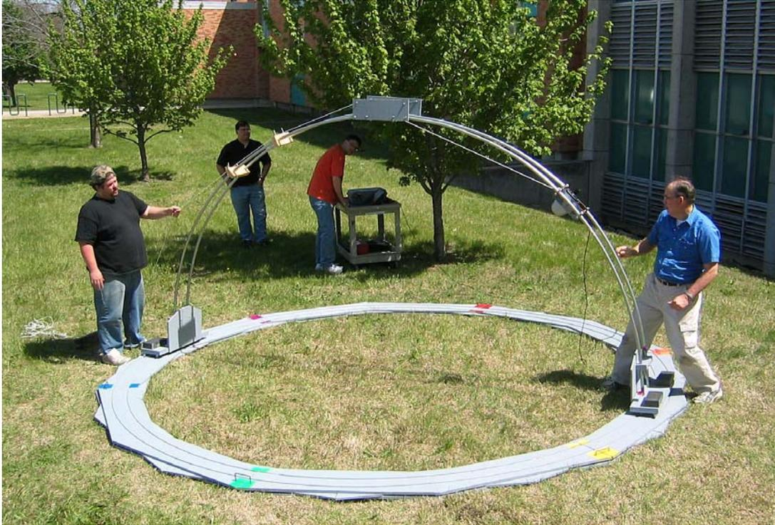
Figure 8. Goniometer ready for field testing outside Science Hall on campus of Emporia State University. A portable computer is connected to the radiometer and is positioned under a nearby tree for shady operation.
