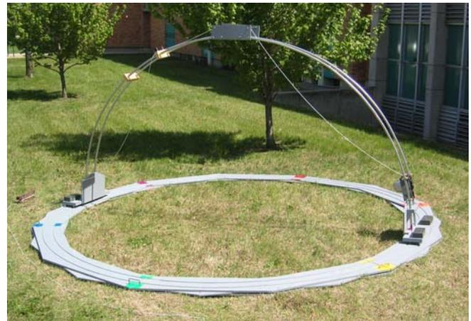
Figure 7. Fully assembled goniometer. Lead weights hold the arch carriages in their tracks. Shadows cast by the arch are minimal.
